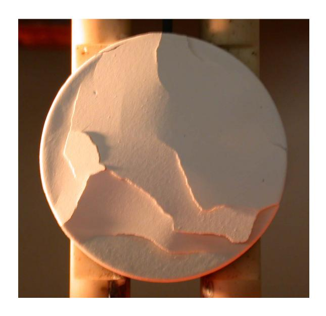
Figure 1.3: TBC spallation due to buckling after thermal cycling.
